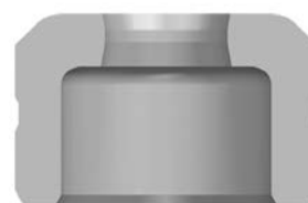
System E :3 cuts with different angles ensures the locking of the slug.
