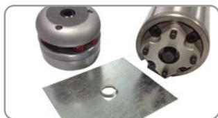
OPTION 2 B station single extrusion 1 hit up forming
