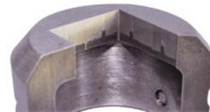
Lock slug AS best option when thickness > 3 mm.
