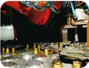
Wire EDM load-unload cell.
